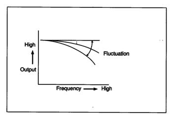
With the Dolby HX PRO system, the effective bias amount added to the bias current is controlled in millisecond units to greatly reduce distortion, improving linearity in high-range response and ensuring high-intensity recording with minimal distortion and noise.
