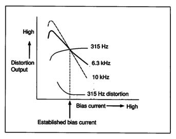
As shown above, characteristics such as output level and distortion differ widely according to the bias (high-frequency) current. In conventional systems, the bias current is susceptible to variations in certain recording signals (see diagram below) which may cause fluctuations in frequency response, distortion, or other unwanted characteristics.
